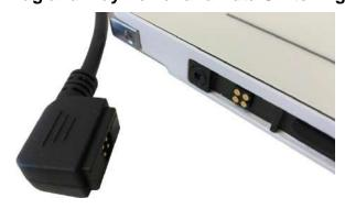
With the flexible design of our Panels it is possible to switch between different operation modes by plug and play. Simply unplug the TCP/IP Data cable to use the panel wireless and vice versa without a need of a new configuration of the device. A magnetic connector for the power plug ensures easy online switching between line operation and battery operation. This enables a fast change between fixed place and mobile mode operation of the panel.
